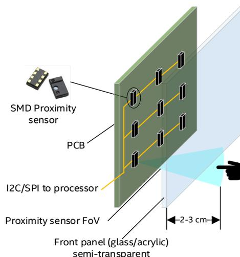
**Figure 1. Conceptual non-touch IR proximity sensor-based keypad solution**
