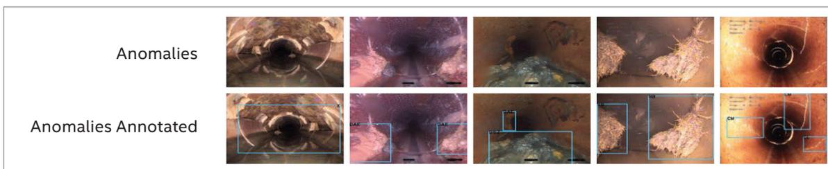
Figure 1. Sample anomalies and annotated images using the Pipe Sleuth solution.
